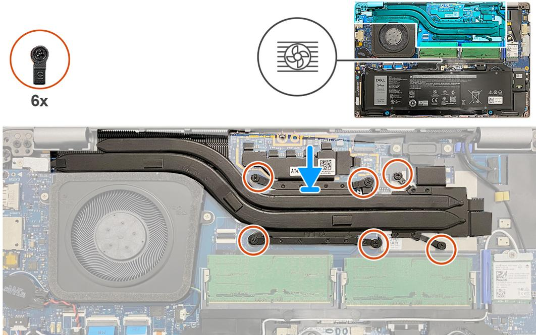
Figure 28. Installing the heat sink
