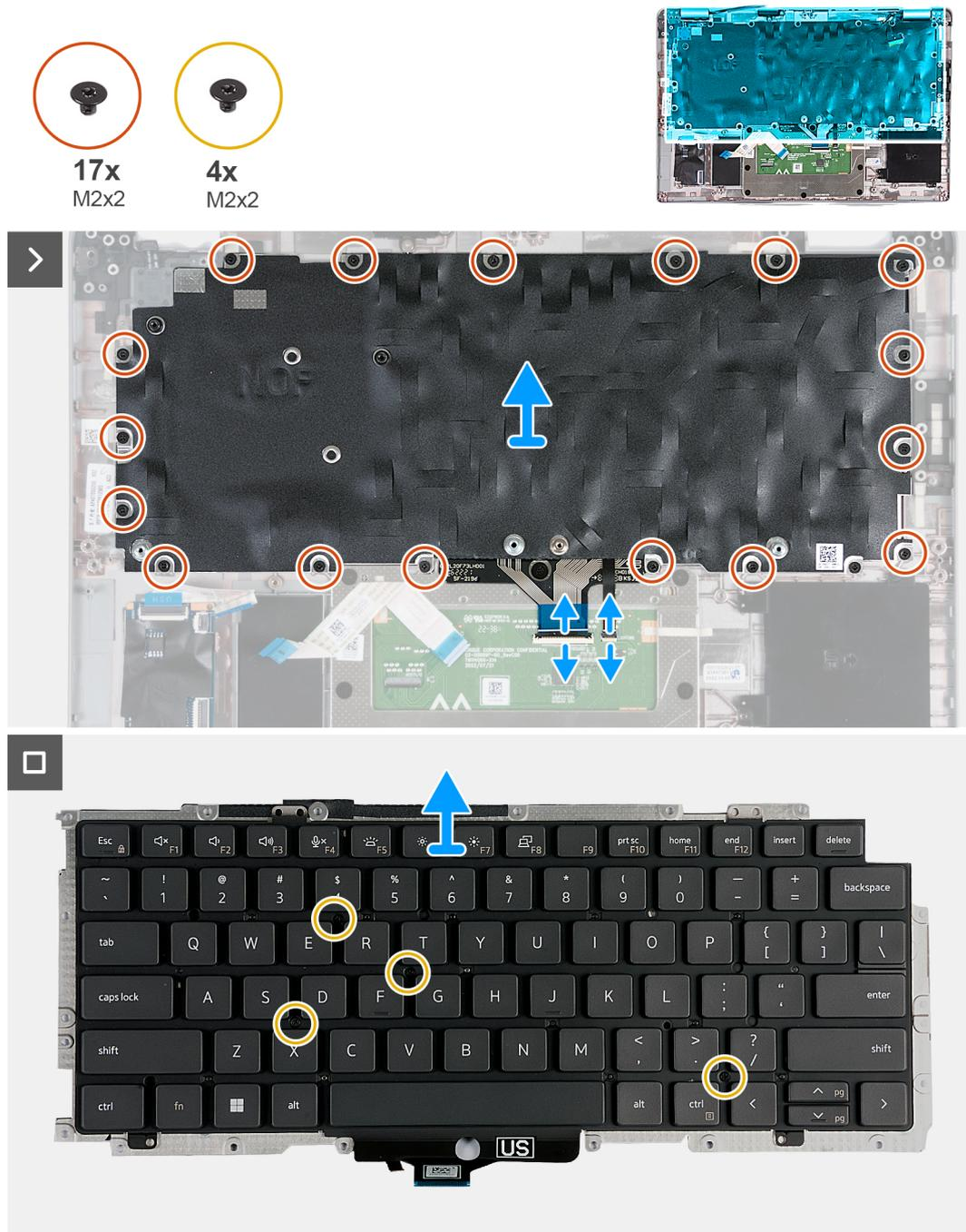
**Figure 61. Removing the keyboard**
