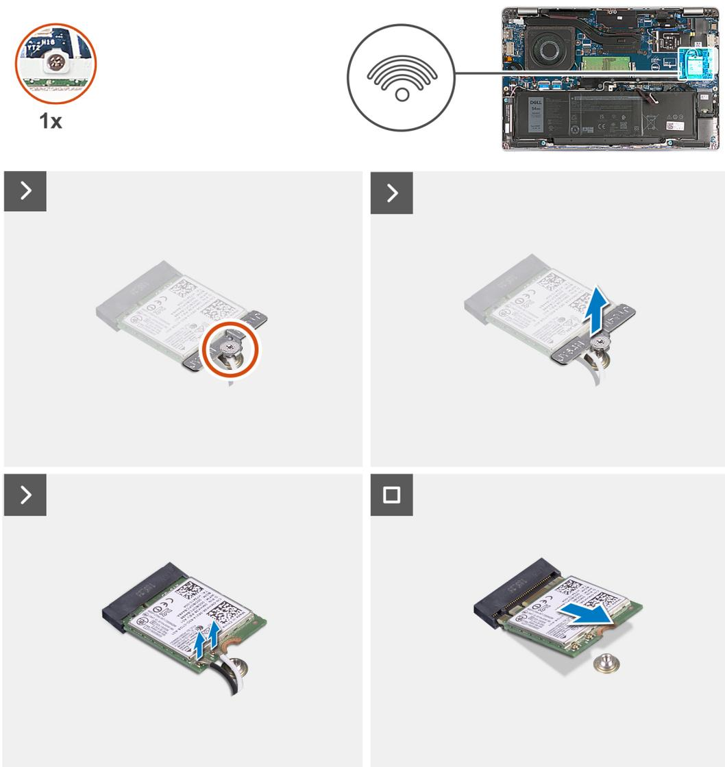
**Figure 10. Removing the wireless card**
