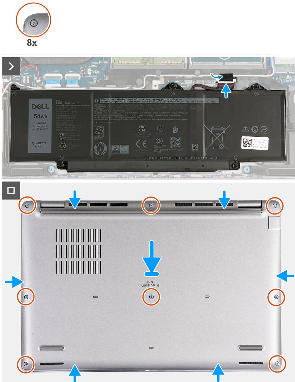
Figure 5. Installing the base cover
