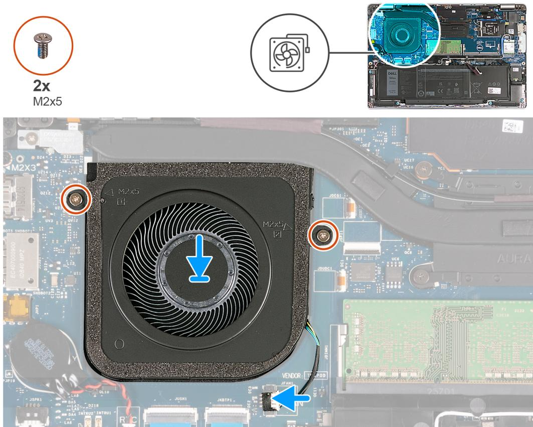
**Figure 17. Installing the fan**
