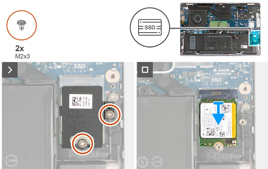
Figure 8. Removing the M.2 2230 solid-state drive
