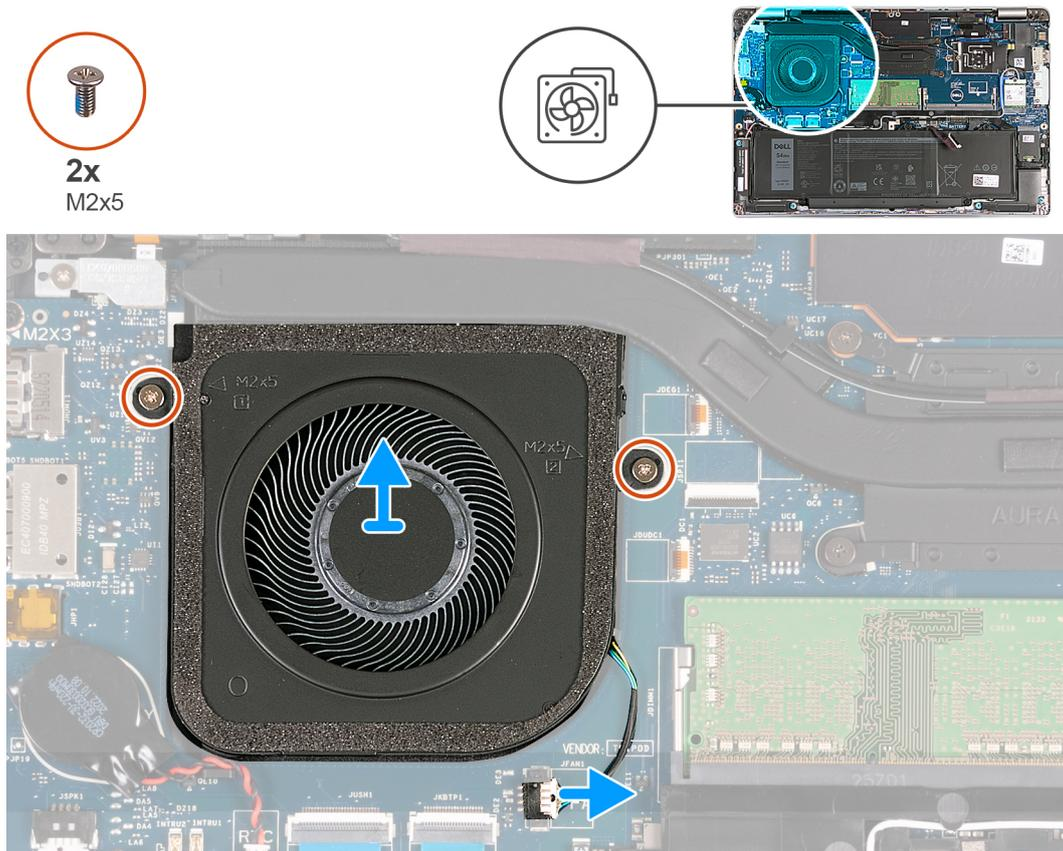
**Figure 16. Removing the fan**
