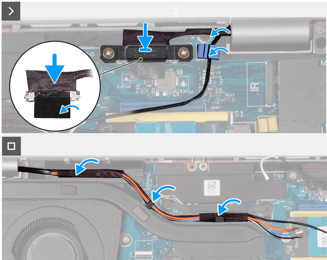
**Figure 40. Installing the display assembly - For computers shipped with 5G card**
