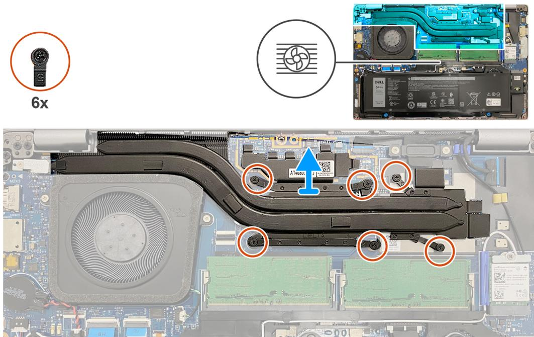
Figure 27. Removing the heat sink
