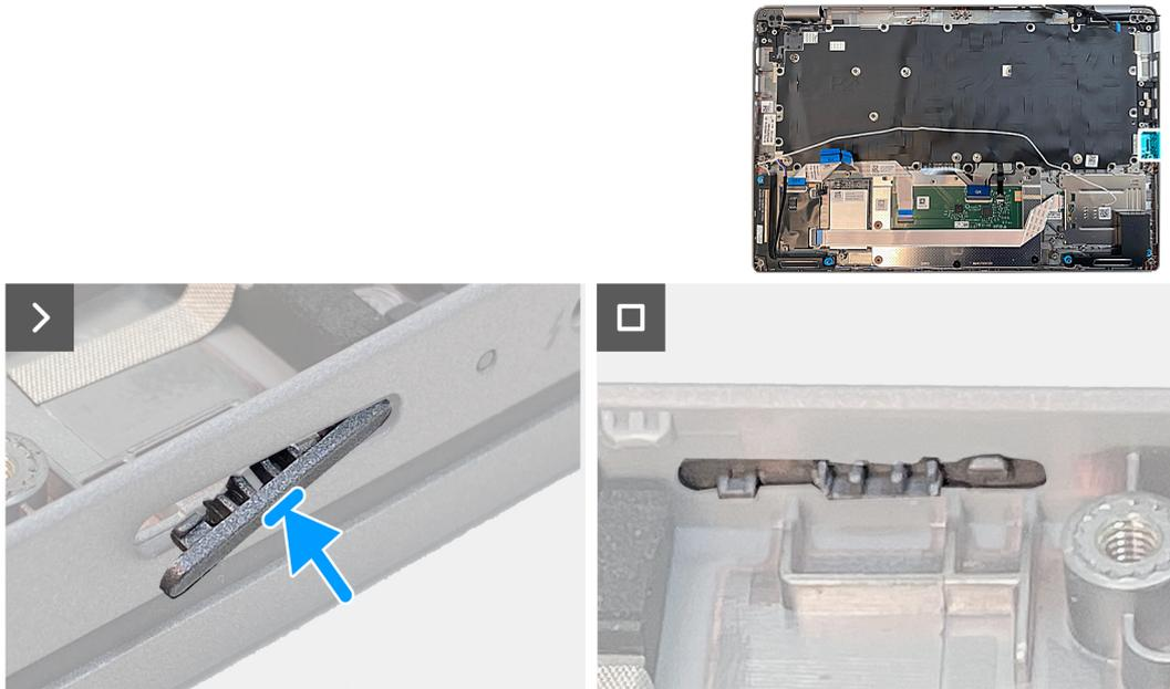
**Figure 66. Installing the dummy SIM-card slot filler**
