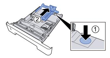
2 Adjust the position of the paper width guides located on the left and right sides of the cassette. Press the paper width adjusting tab and slide the guides to the paper size required.
