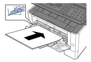
Insert the paper along the paper width guides into the tray until it stops.
