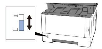
Remove the paper from the cassette once if there is no improvement, turn it over and reload it, or change the loading direction by rotating the paper 180 degrees.
