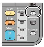
If print data is received during Sleep, the machine automatically wakes up and starts printing.
