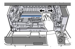
7 Slide the charger cleaner knob on the upper side of the drum unit left and right 2 or 3 times.
