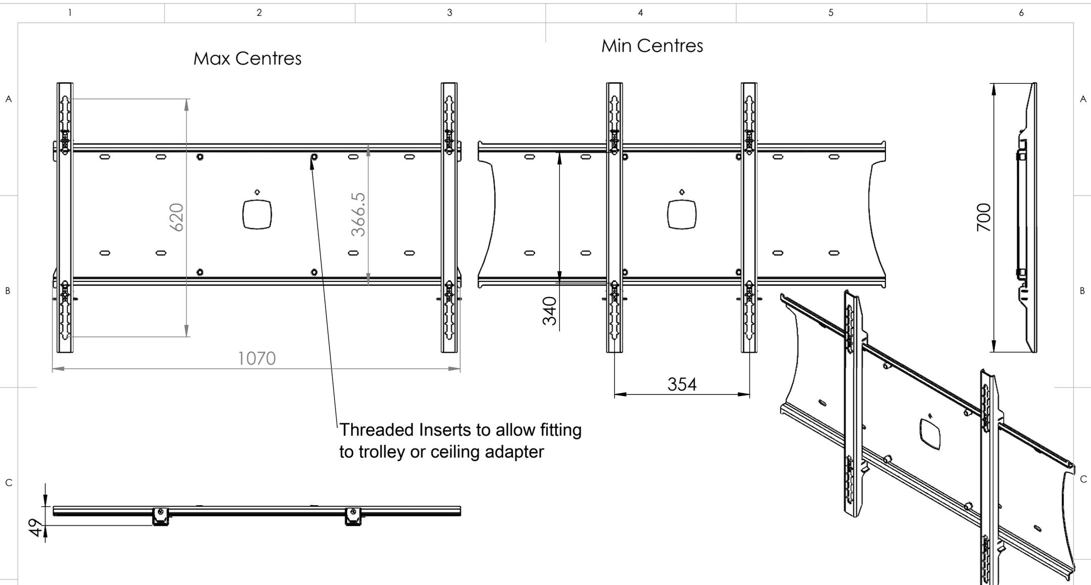
Threaded Inserts to allow fitting to trolley or ceiling adapter
