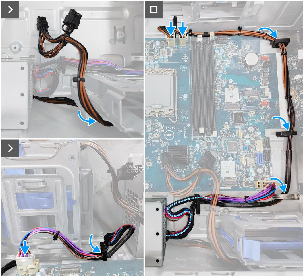
4. Connect the power cables to the connectors on the system board.
