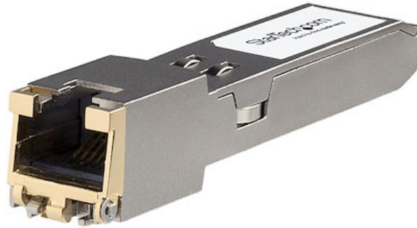
The JL563A-ST is a HPE JL563A compatible copper transceiver module that has been designed, programmed and tested to work with HPE brand switches and routers. It delivers dependable 10 GbE connectivity over copper cable, for 10/100/1000/10000 compliant networks, with a maximum distance of up to 30 m (98.4 ft).
