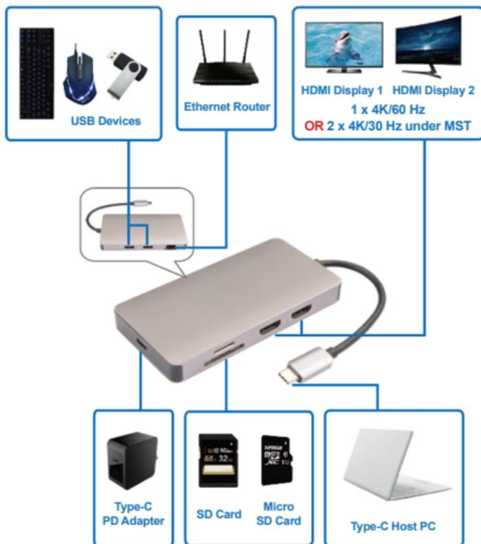
**Note:** When connecting to a DP 1.4 Alt Mode supported host, the max resolution of the HDMI ports is 4K/60 Hz (Dual: 4K/30 Hz). If connecting to a DP 1.2 Alt Mode supported host, the max resolution of the HDMI ports is 4K/30 Hz (Dual: 1080p/60 Hz) due to the limited bandwidth.
