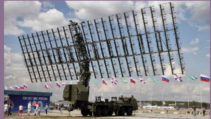
1L119 Nebo-M meter-band VHF '3D' AESA
