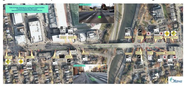
The lanes would be delineated with both Super Sharrows and diamonds painted on the road surface. In addition, there would be other pavement markings further demonstrating it was for the exclusive use of bicyclists and buses. In Figure C, a green stripe down the centre of the lane is shown as a possible lane marking. Staff would also consider hatched lines.
