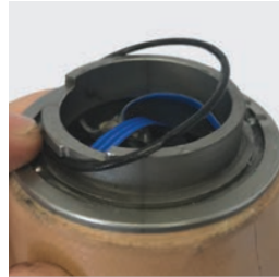
Installing lubricated O-ring.
