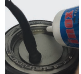
Applying lubricant to groove.
