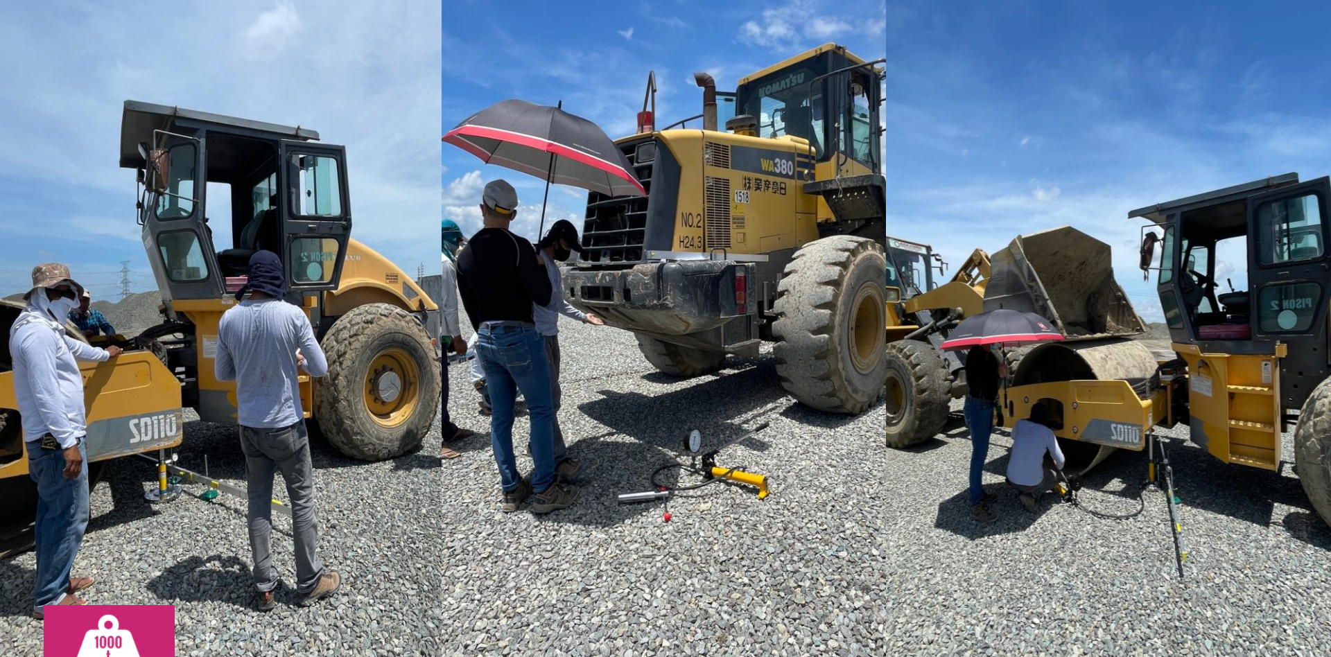
Ground Improvement | Plate Load Test BS EN 1377 Part 9:1990 | Philippines
