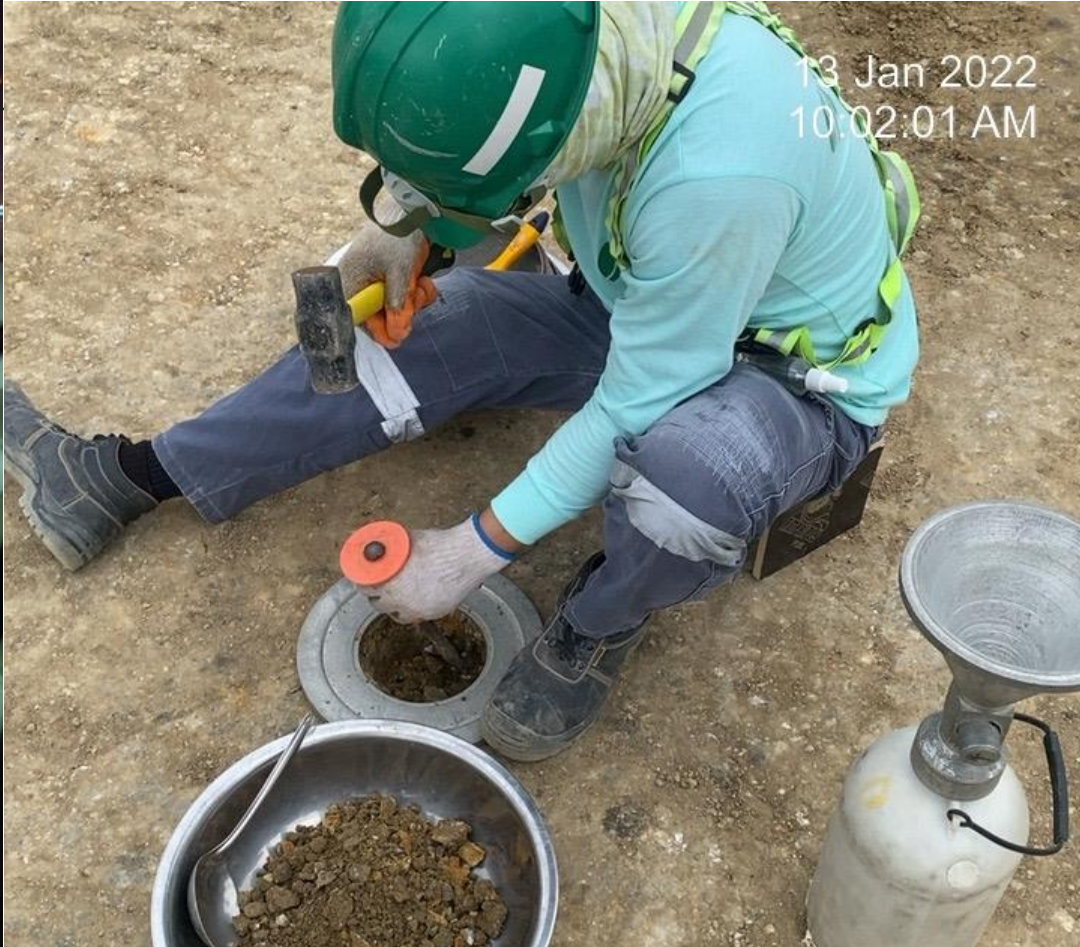
Ground Improvement | Field Density Test (95% MDD) | Batangas, Philippines
