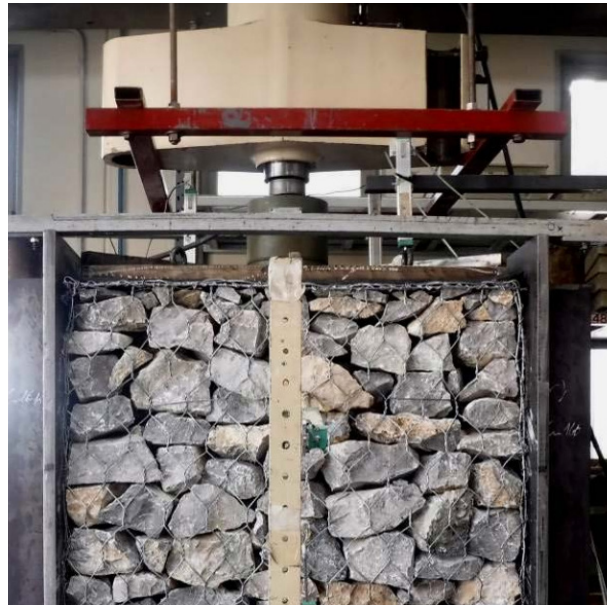
Full Scale Compressive Test
