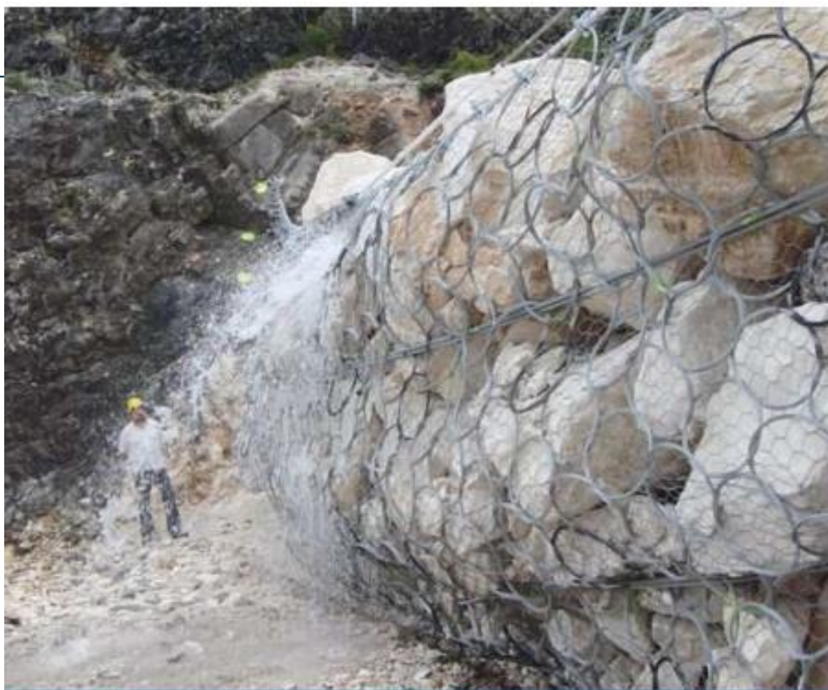
Fig. 4: Full-scale test on RMC DF barrier
