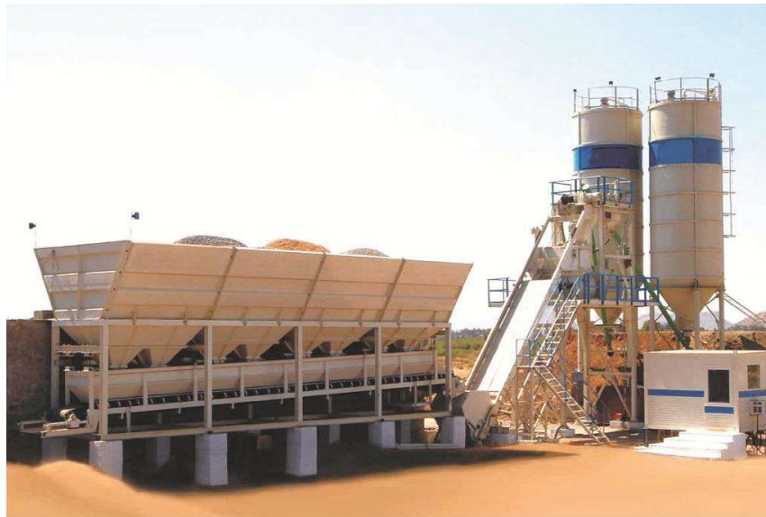
Concrete Batching Plant (photo taken from gharpedia.com)
