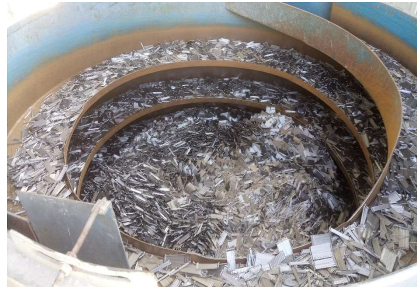
Steel fibre doser machine / aggregate bin
