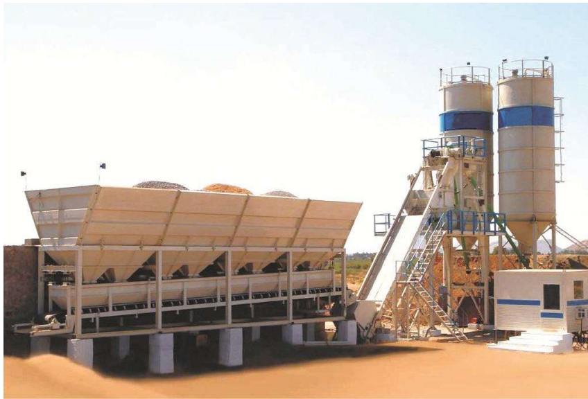
Concrete Batching Plant (photo taken from gharpedia.com)
