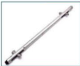
Stain gauge, inclinometer, etc. Equipped with radio transmitter "SFL"
