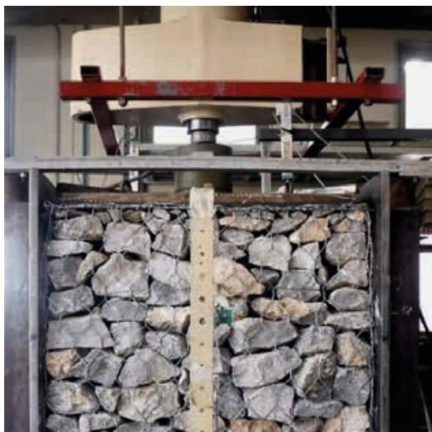
Full Scale Compressive Test
