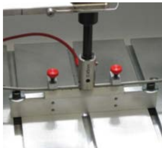
ABRASION TEST - ASTM A975-21
