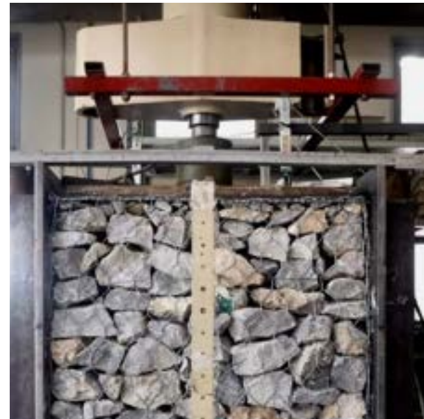
Full Scale Compressive Test
