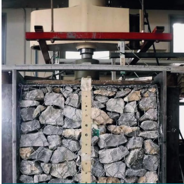
Full Scale Compressive Test
