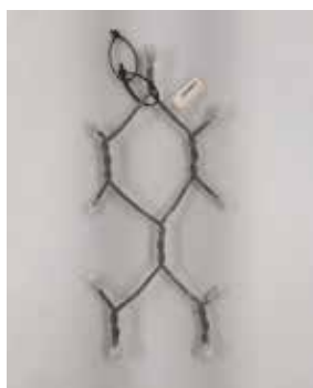
Test Specimen, before and after Salt Spray Test (ISO 9227)
