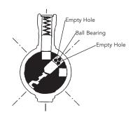
Shown above is a cross section of a 21-Option Lost Ball Cylinder with the Construction Master Key inserted and rotated.
