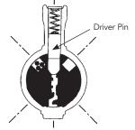
If the Construction Master Key is inserted (as shown) after being voided, it will not rotate because Driver pin now extends into the plug chamber. This prevents it from rotating and voids the Construction Master Key.
