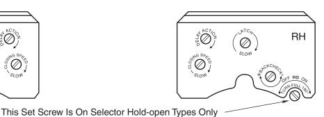
Closing speeds can be adjusted to suit local conditions and requirements. Label on closer face designates the purpose of each adjustment screw. Adjustments are for speed control.
