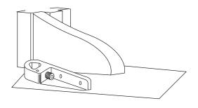
CAUTION: Closer is shipped with "valve" screws down. DO NOT FORCE VALVE DOWN.
