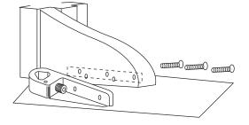
CAUTION: Closer is shipped with "Stroke" valve down.
