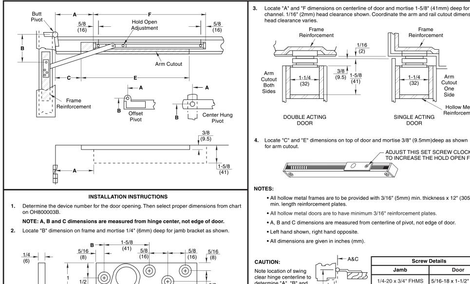
channel. 1/16" (2mm) head clearance shown. Coordinate the arm and rail cutout dimensions if head clearance varies. Frame Frame Reinforcement Reinforcement 1/16 (2) 3/8 Arm 1-5/8 (9.5) Arm 1 - 1/4<u>1-1/4</u> Cutout (41)(32)Cutout (32) Both One Sides Side
