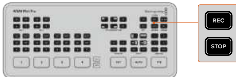
Press the record button, marked 'rec', to record your broadcast to an external drive or flash disk via USB-C
