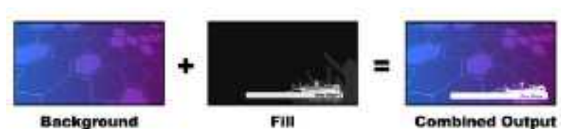
Combining a background and fill/key in a luma key
