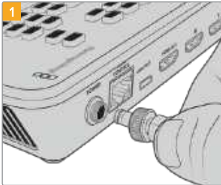
1 Connect power to ATEM Mini's power input using the supplied cable
