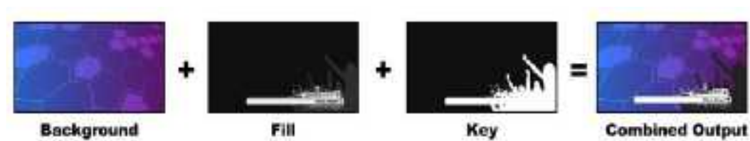
Combining a background, fill and key in a linear key
