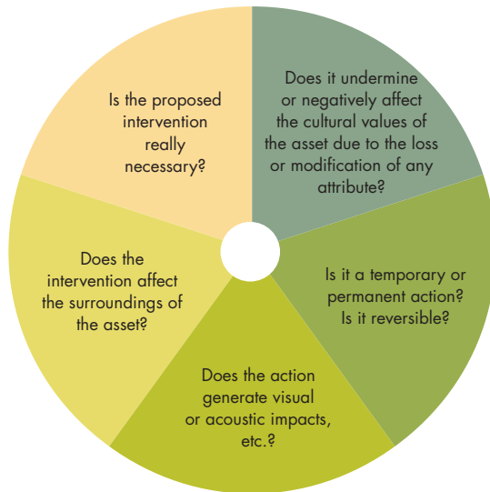
Example of issues to be assessed in a proposal for intervention on cultural heritage
