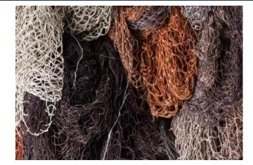
Aquafil regenerates fishing nets and other nylon waste (e.g. textile production scraps) into a new yarn, having the same characteristics as nylon made of virgin raw material called ECONYL<sup>®</sup>.
