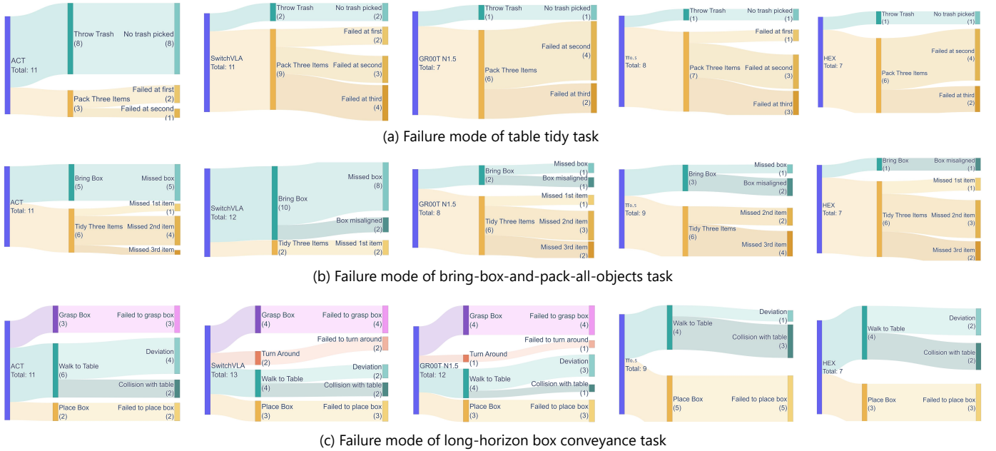
Fig. 8. Failure analysis across different methods and tasks. Each Sankey diagram shows how failed trials are distributed across task stages and fine-grained error types, with flow width proportional to the number of failures.
