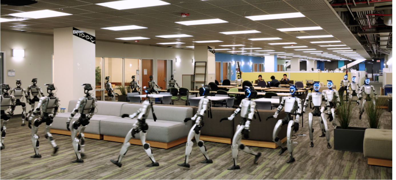
Fig. 1: Long-Horizon Humanoid Navigation in Cluttered Scenes. We propose TANGO, a whole-body foundation model for cluttered indoor scene navigation. TANGO demonstrates strong scene understanding and robust traversal capability, navigating a 30-meter route zero-shot in a real-world cluttered office scene.
