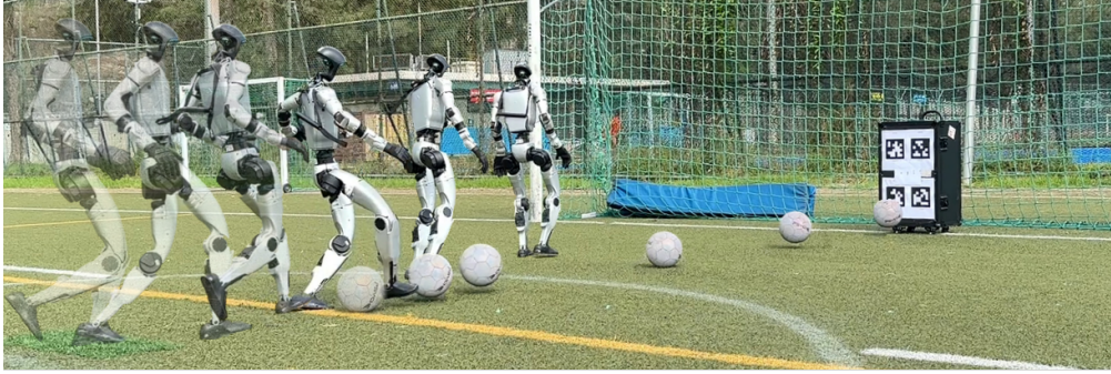
Figure 1: RoboNaldo: accurate, stable and powerful whole-body soccer shooting on a real grassy soccer field. Ghost-overlaid time sequence of a Unitree G1 humanoid executing a directed penalty kick.
