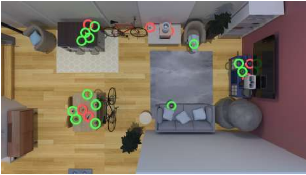
Fig. 9. Spatial Distribution of Success and Failure. Green and red circles represent successful and failed grasping attempts, respectively.
