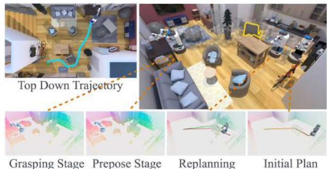
Fig. 1. Visibility-Aware Mobile Grasping. A mobile manipulator approaches a target while a chair appears in its path.
