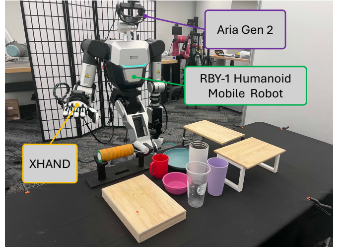
Fig. 6: Hardware setup. We evaluate on a Franka tabletop setup with an Intel RealSense D435 and an RBY-1 humanoid mobile robot with ROBOTERA XHAND and Meta Aria Gen 2 glasses.
