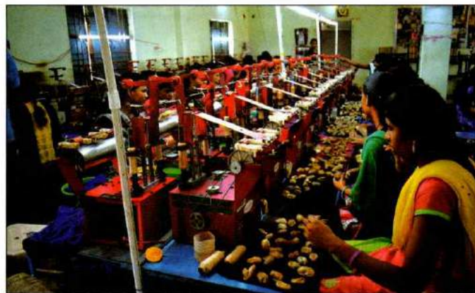
Employees working on solar silk reeling machines manufactured by Resham Sutra at a reeling centre in Odisha.
