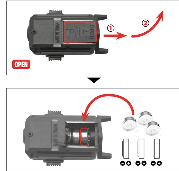
Insert batteries. (Mind their polarities!) Close battery compartment.
